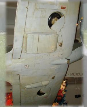
Specific to the early marks of Spitfire are the radiator fairing and the smaller oil cooler housing that sit under the wing. We recovered both from AA810 but only the radiator fairing has salvageable parts within it.
