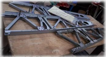
Rib sections are complicated with most parts being individual to each assembly. Great care is taken to restore each useable part to retain a high level of originality.
