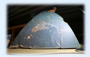
One original top skin will be kept for display but the internal structure and the remaining skins will be able to be used after careful restoration.
